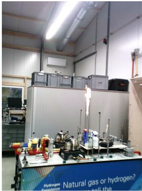
A test set-up with natural gas and hydrogen flares: with a visual camera, the hydrogen flares are not or hardly visible. However, a thermal imaging camera can visualize them based on the thermal radiation the hydrogen flares emit.
