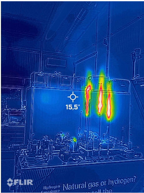
A test set-up with natural gas and hydrogen flares: with a visual camera, the hydrogen flares are not or hardly visible. However, a thermal imaging camera can visualize them based on the thermal radiation the hydrogen flares emit.
